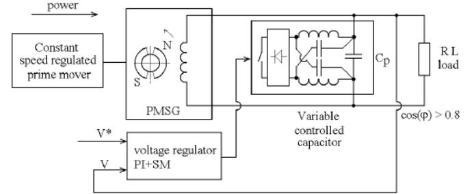
Fig. 10. Three kW, 3000 rpm, 50 Hz, 1 phase a.c. PM generator with step capacitor  $\pm 5\%$  voltage control down to 0.8 lagging power factor loads [15].
