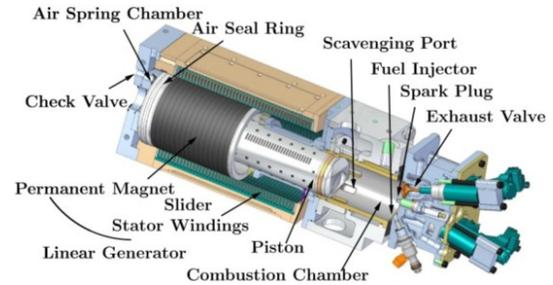
(a)generator driven by linear thermal engine
