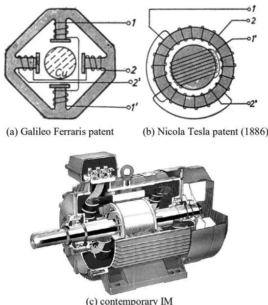
Fig. 1. Induction motors. (a) Galileo Ferraris patent;(b) Nicola Tesla patent (1886); (c) contemporary IM
