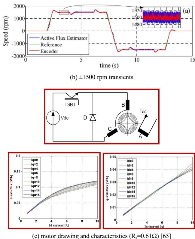
Fig. 15. Relsyn motor encoderless drive with active – flux – based flux oriented control from zero to 3000 rpm: (a) zero speed operation with 1 Nm full torque; (b)  $\pm 1500$  rpm transients; (c) motor drawing and characteristics ( $R_s=0.61\Omega$ ) [65].
