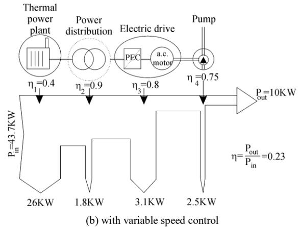
Fig. 3. Energy flow from fossil – fuel power plant to electric motor pump: (a) with valve offering flow rate control, (b) with variable speed control
