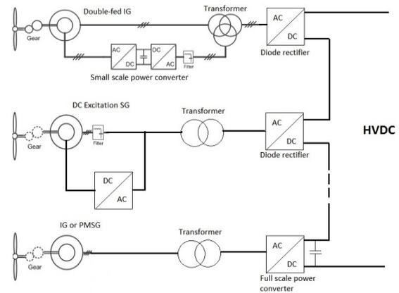
(b) DFIG DC excited SG with variable frequency, PMSG (IG) with variable frequency
