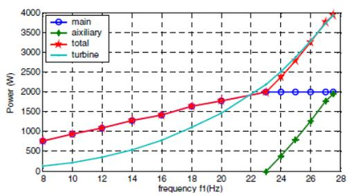
(b) dual stator winding CRIG with d.c. output [13]
