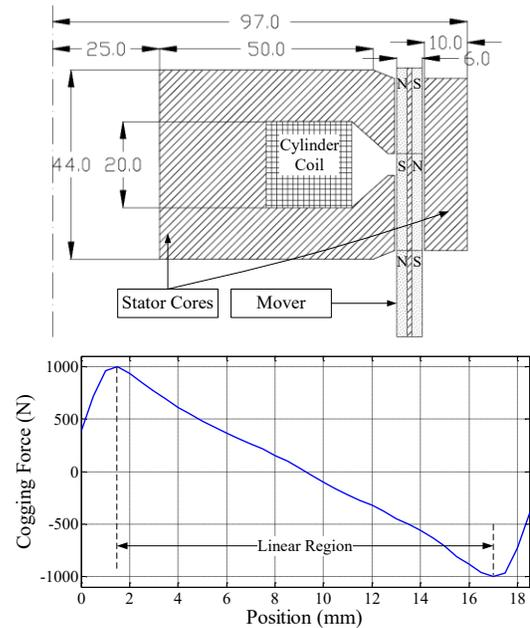
(b) potential springless resonant device with PM mover and magnetic (cogging) “virtual spring” [67]
