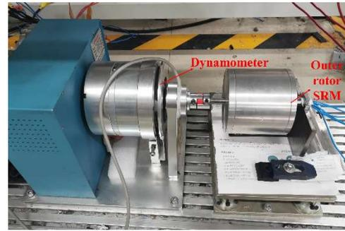
Fig. 14. Photo of the experimental platform
